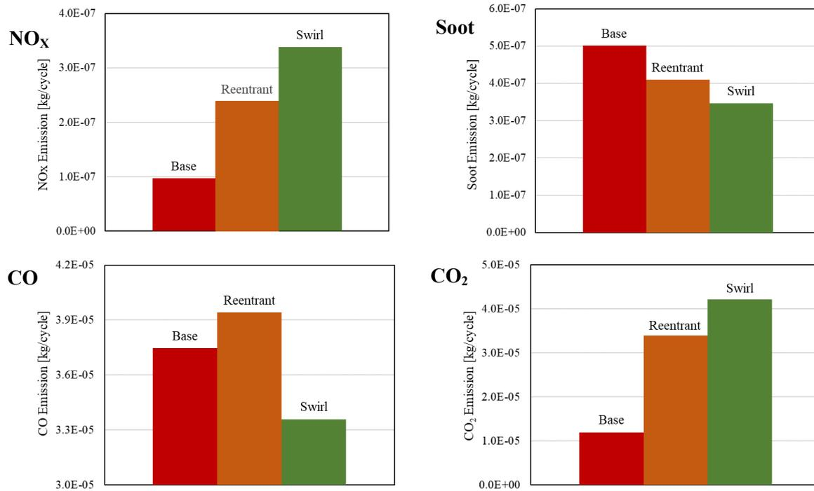
**Figure 6.** Exhaust emissions of three different piston bowls.
