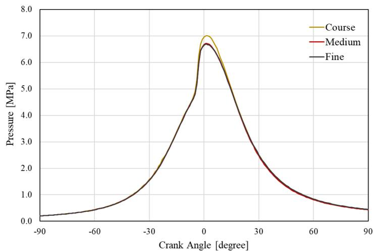
**Figure 3.** In-cylinder pressure curves of the mesh independency studies.
