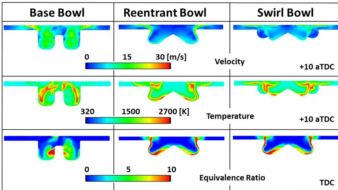
Figure 5. In-cylinder velocity, temperature, and equivalence ratio distributions of three different piston bowls.
