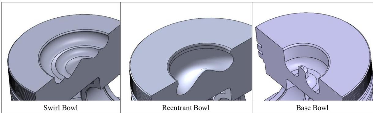
**Figure 1.** Geometries of the different piston bowls.
