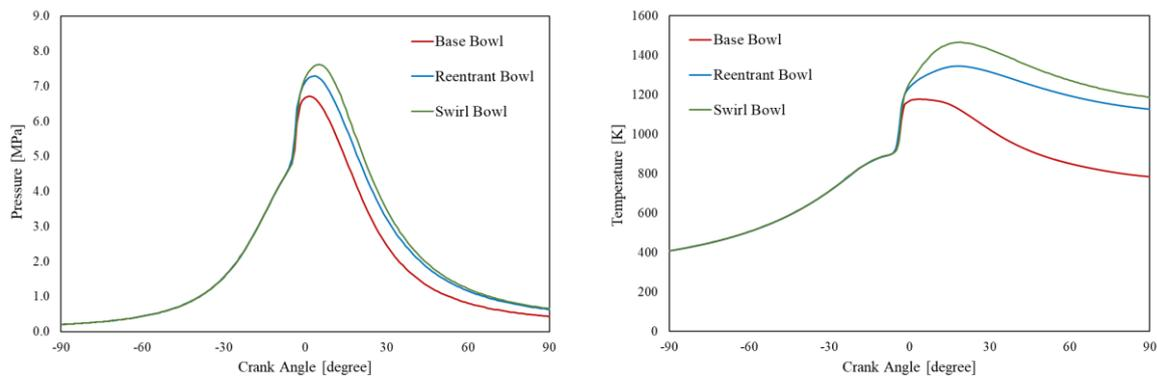
Figure 4. In-cylinder pressure and temperature curves for three different piston bowls.
