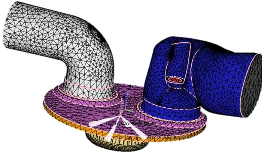
**Figure 2.** The surface of the CFD model at TDC with baseline piston bowl.
